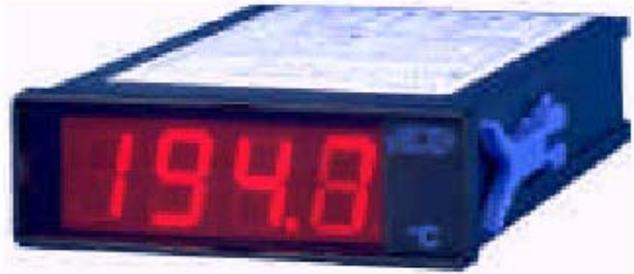
Digital panel meters TNE2 can be used with temperature sensors. Temperature is displayed in °C. Those industrial apparatus are automatically delivered with a removable screwing connector, and an analog output. The large readable display is made of red LED (green or yellow in option)
