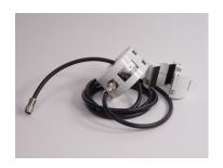
Frequency Range: 1 MHz – 400 MHz Insertion Loss: 4 to 22 dB Transfer Impedance: 12 to 33 dBΩ Rated Watts: 100 watts CW Connector: N-Type, female
